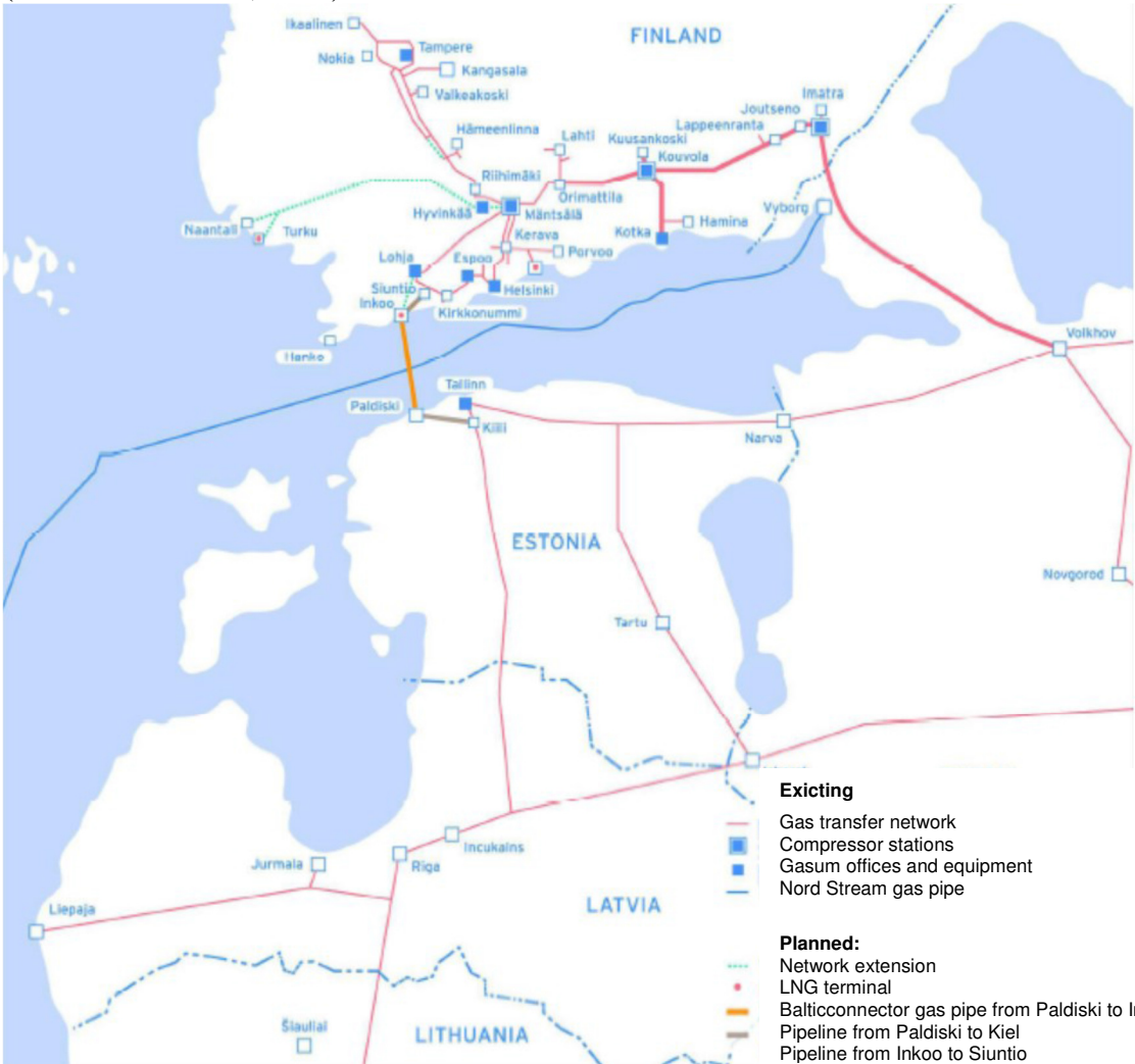
Figure 2.2. Gas pipes in the Gulf of Finland region (existing and planned) (Ramboll Eesti AS, 2014).
